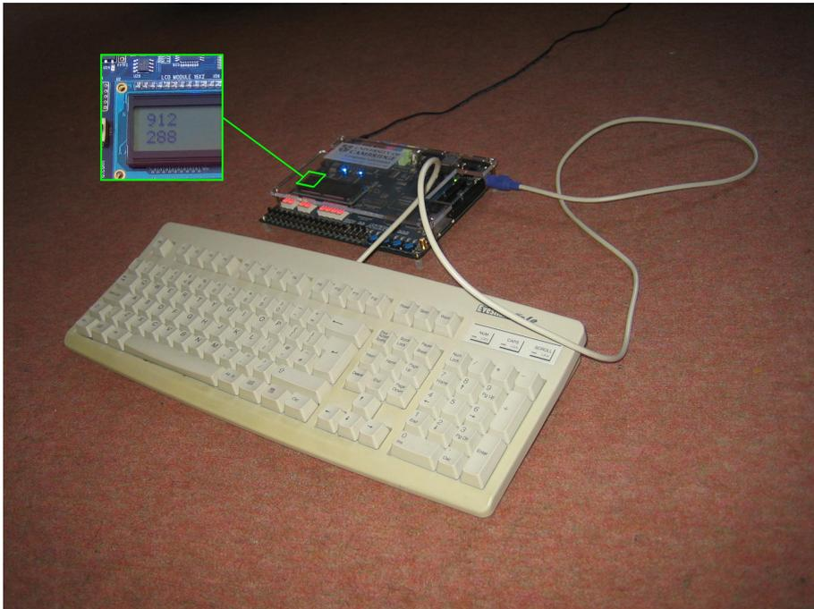
Figure 4.3: Photograph of the DE2 board running the pocket calculator
