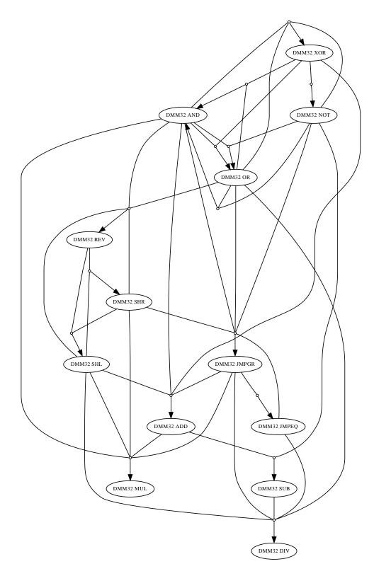
Figure 3.4: Emulation routines available between instructions of DMM32
