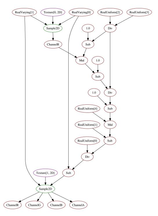
Figure 3.2: Dataflow graph of autostereogram fragment shader.
