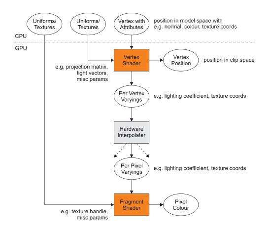
Figure 2.1: The graphical shader pipeline.
