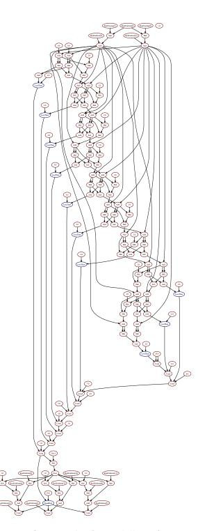
Figure 4.5: Dataflow graph of Mandelbrot fragment shader.
